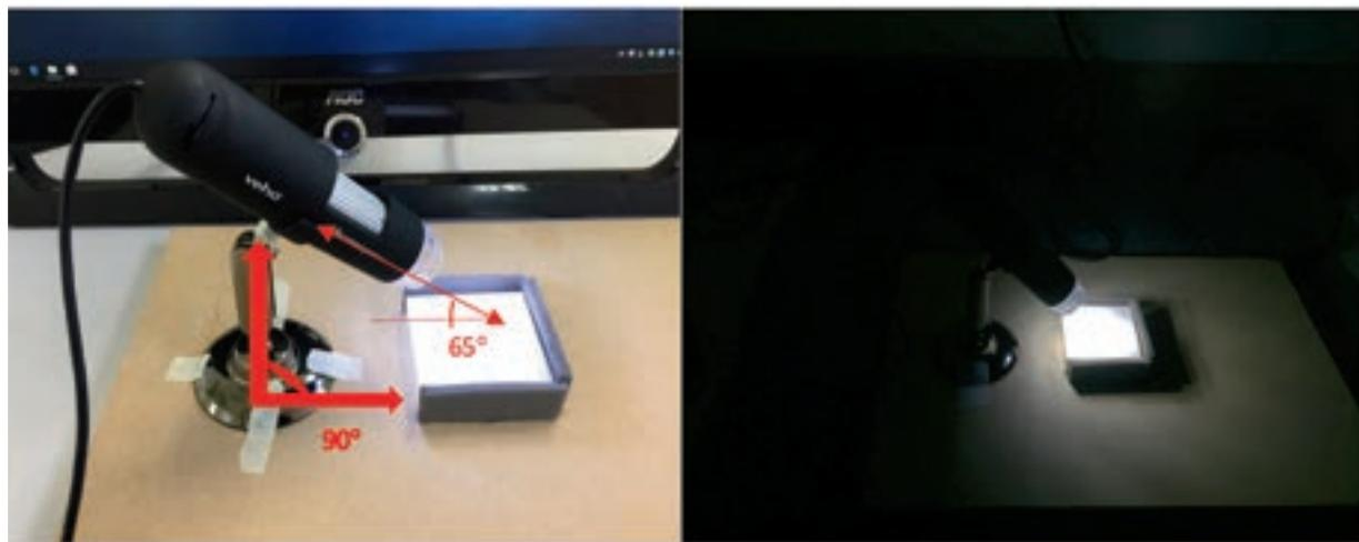
Figure 2: The image on the left shows the microscopy setup and angles in the light. The image on the right shows how the samples were photographed in the darkroom. Photo: Amanda Berg.
