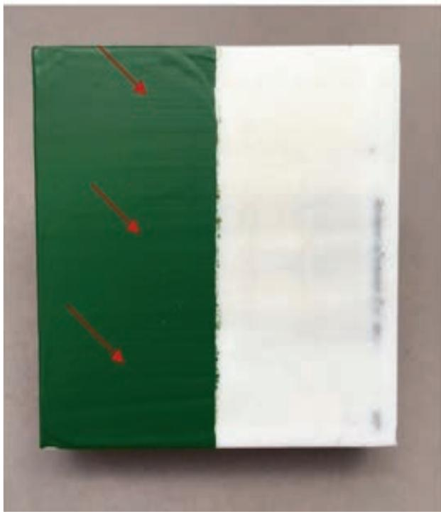
Figure 5: This image shows a PLA sample processed by abrasion with paint applied and the corrugation visible through the paint. Photo: Amanda Berg.
