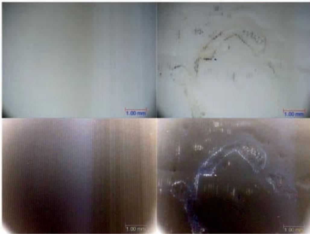
Figure 6: Photomicrograph showing an ABS sample processed by heat. Some discolouration and warping can be seen. Photo: Amanda Berg.
